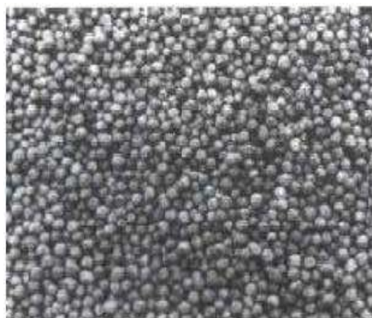
Figure (I.3) : structure non consolidée [2].
