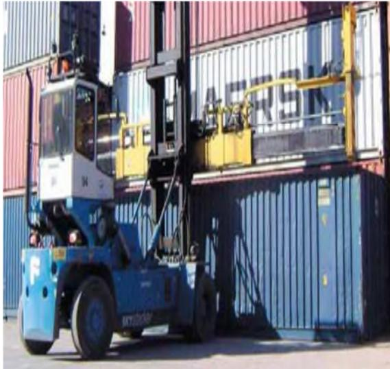
**Figure 36 :** Front Loaders (Spreaders).
