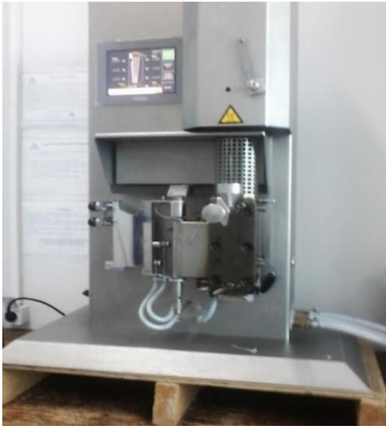
Figure 21: Extrudeuse bis-vis de type DSM Xplore.
