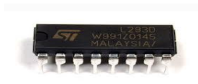
Fig.3. 6. Le circuit L293D. [33]
