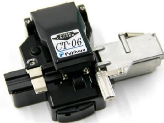
Figure I.14: Cliveuse fujikura CT-06
