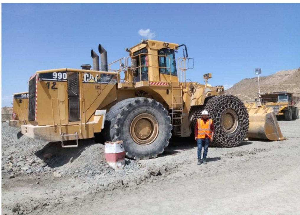
Figure. (II.7) : Chargeuse CATERPILLAR 990II.
