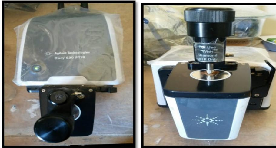
**Figure I.16:** Agilent Technologies CARY 630 FTIR.
