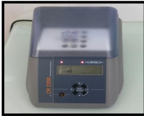
**Figure I.8:**Réacteur DCO.
