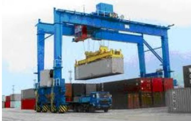
FIGURE 1.4: Rubber-Tyred Gantry Crane (RTGC)
