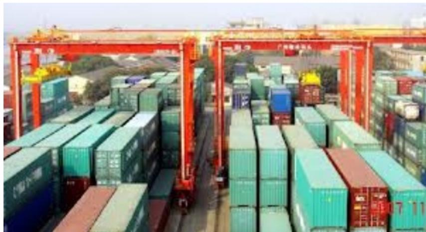
FIGURE 1.3: Rail-Mounted Gantry Crane (RMGC)
