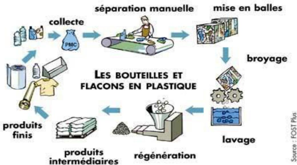
Figure 4 :SCHEMA GENERAL DU PROCESSUS DE RECYCLAGE DU PLASTIQUE
