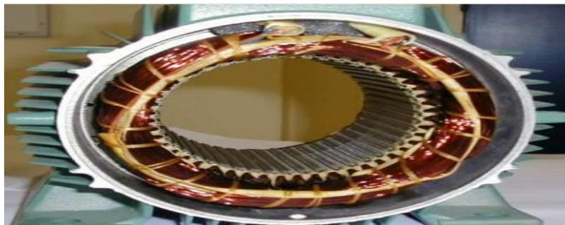
Figure I.4 : Stator.
