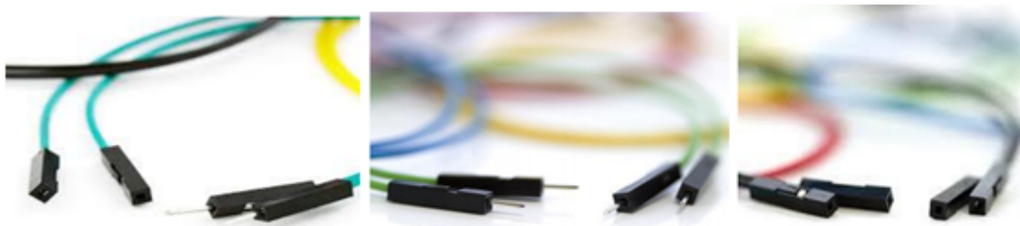
FIGURE III.14 – Fils de raccordement.
