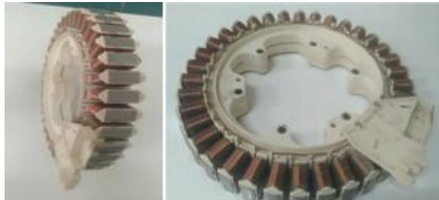
Figure III-6 Stator
