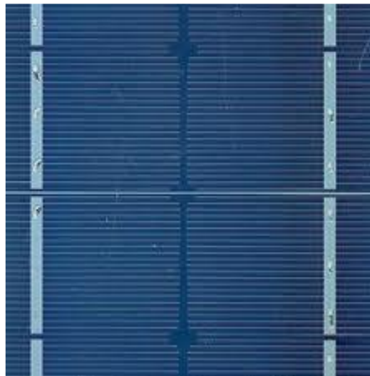
Figure I.5 : Cellules mono- cristallines [18]
