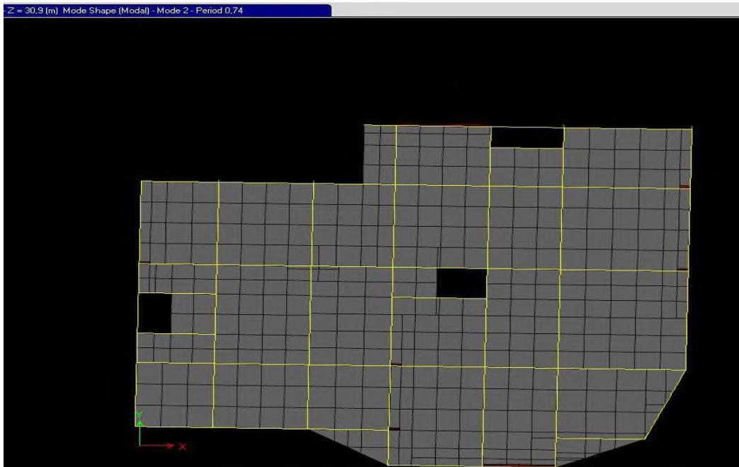
**Figure IV.4** mode 2 T=0,74 sec**3<sup>ème</sup> mode (rotation autour de z) :**
