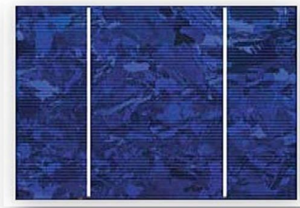
Figure 1.4 : Cellule multi cristallin.
