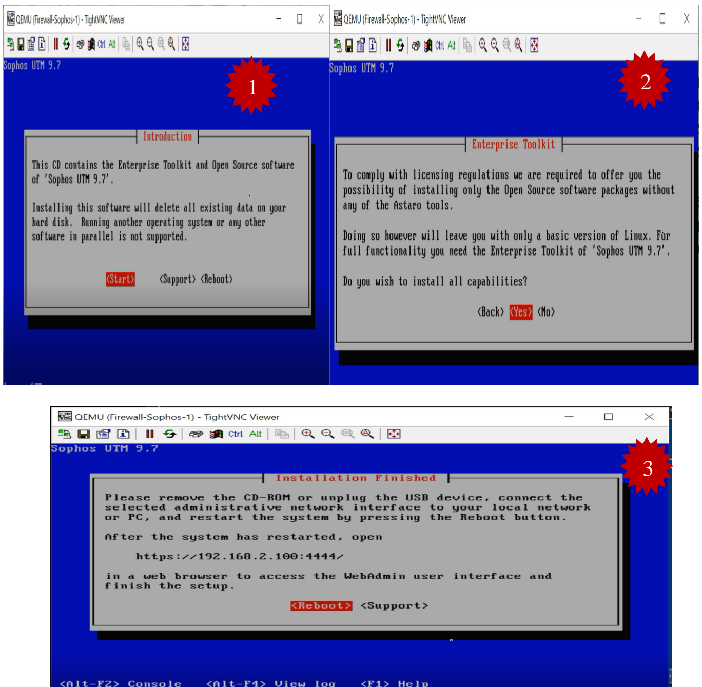
FIGURE IV.66 – Installation Firewall Sophos UTM.
