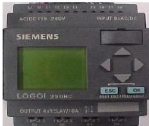
**Figure II.2 :** Automate compact SIEMENS.
