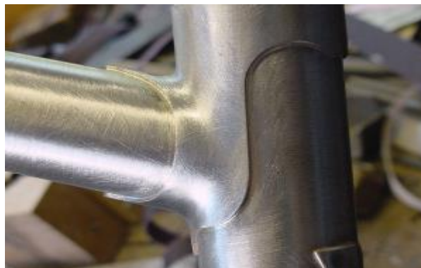
Figure I. 21: Soudage des tubes [3]
