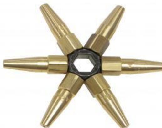
Figure II. 3: Buses de chalumeau [22]
