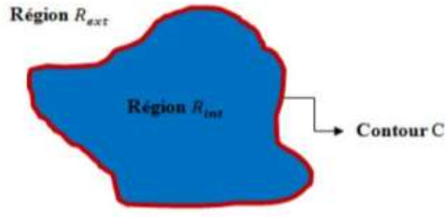
Figure III. 7: Illustration des régions R_{int} =Inside (C) et R_{ext} =Outside (C) de Chan et Vese.
