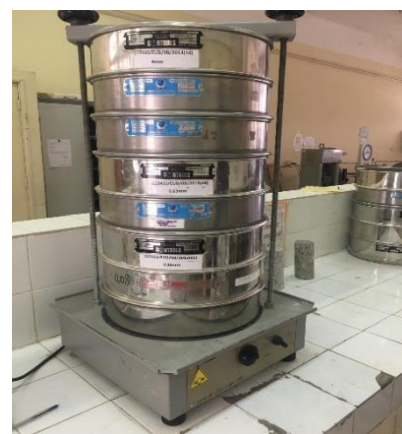
Figure III.8:L'opération de tamisage.
