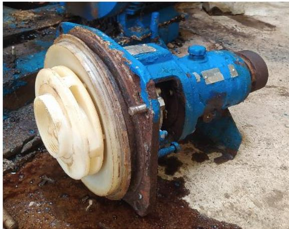
**Figure I.8:** Pompe centrifuge.
