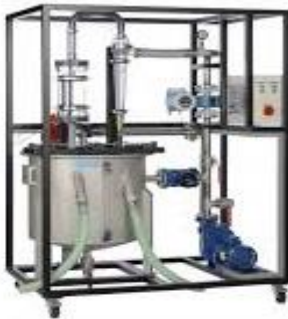
Figure II.13. Hydrocyclone de laboratoire.
