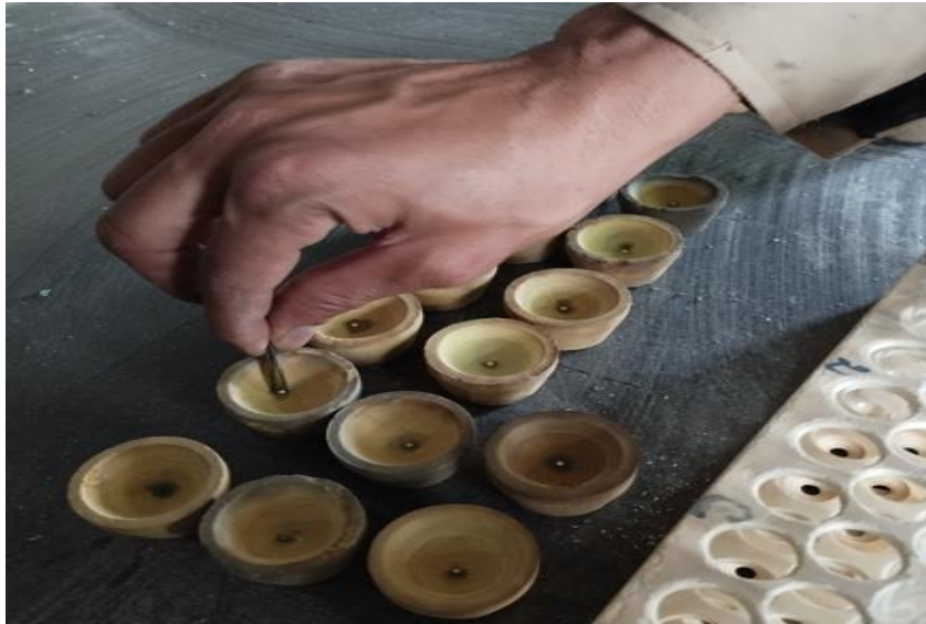
Figure II.14: Coupellation perle or et argent. (Photo prise)
