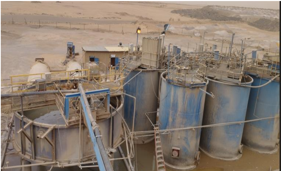
FigureII.29: Les cuves de lixiviation. [Photo prise]
