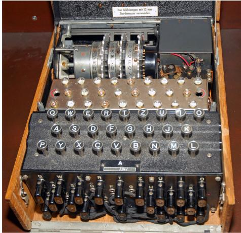
FIGURE 2.4 – Machine Enigma
