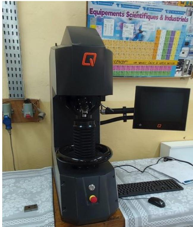
**Figure III. 7 :** durometre type Qness 250 CS
