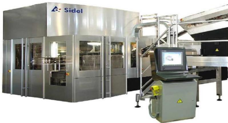
Figure I-2: La souffleuse SBO 10.
