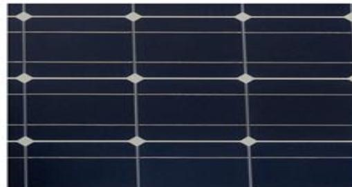
Figure I-2 Cellule de silicium monocristallin [8]
