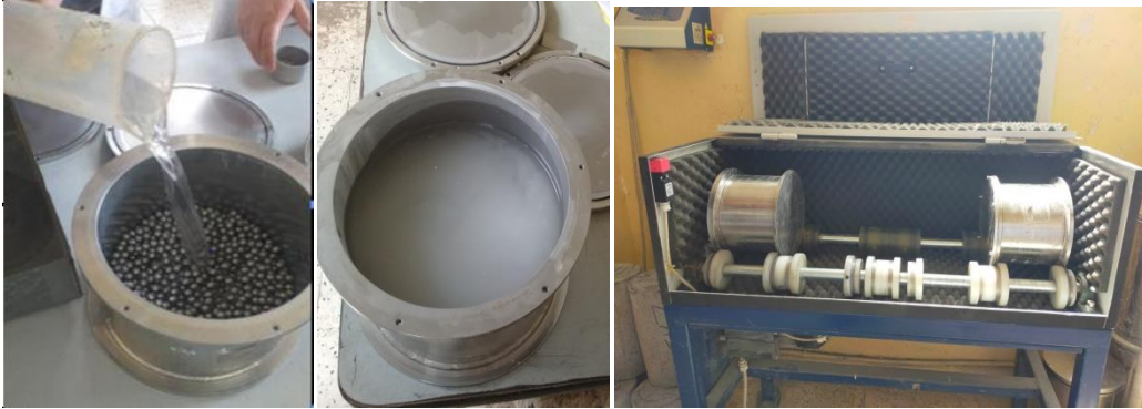
Figure II.8: Appareil de Micro-DEVAL
