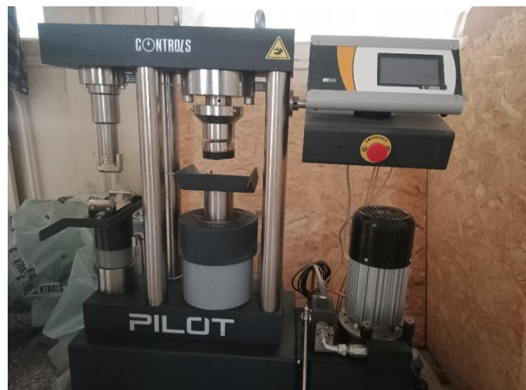
Figure III.7 : Presse hydraulique type CONTROLS PILOT PRO
