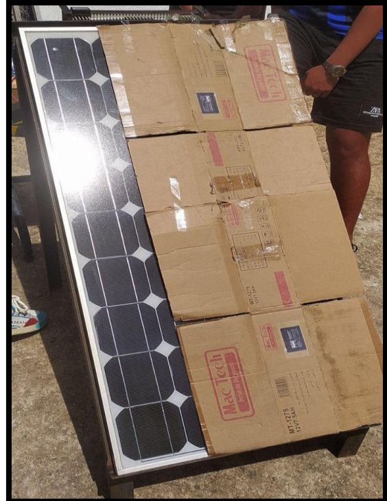
Figure III. 1(b): The solar panel is shaded 68%
