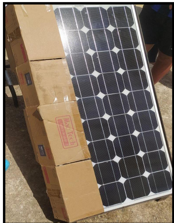
Figure III.1(d): The solar panel is shaded 25%
