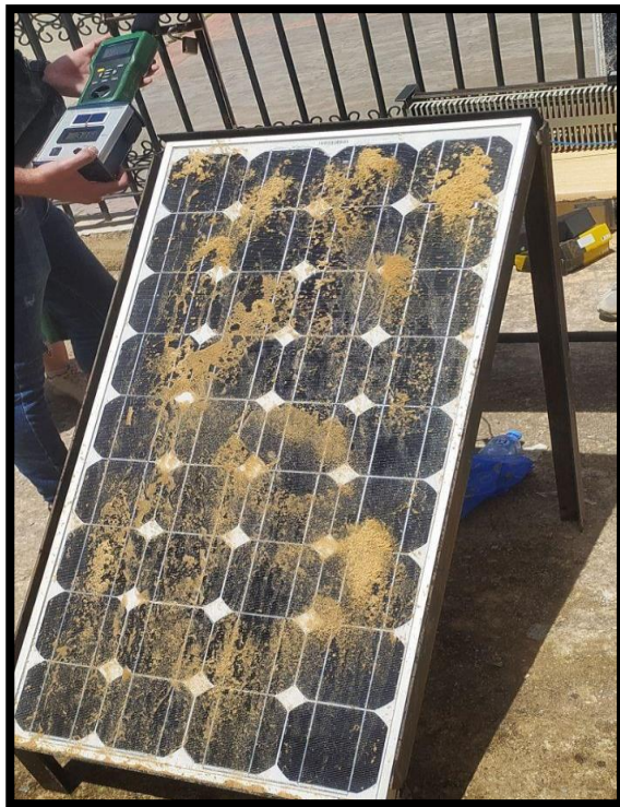
Figure III.1(g): The solar panel is covered with more sand
