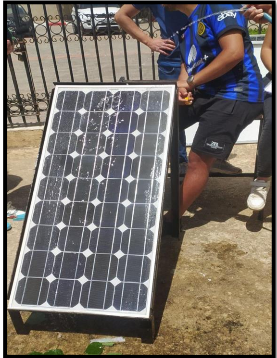
Figure III.1(f): The solar panel is covered with water
