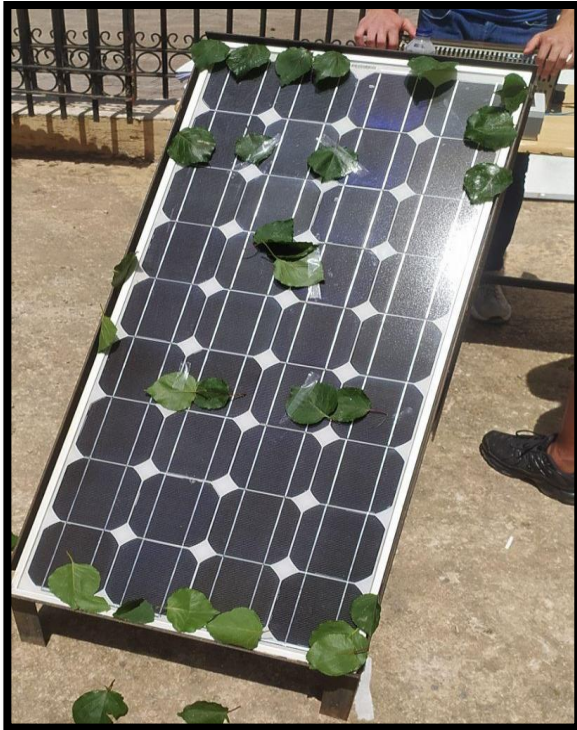
Figure III.1(e): The solar panel is covered with tree leaves
