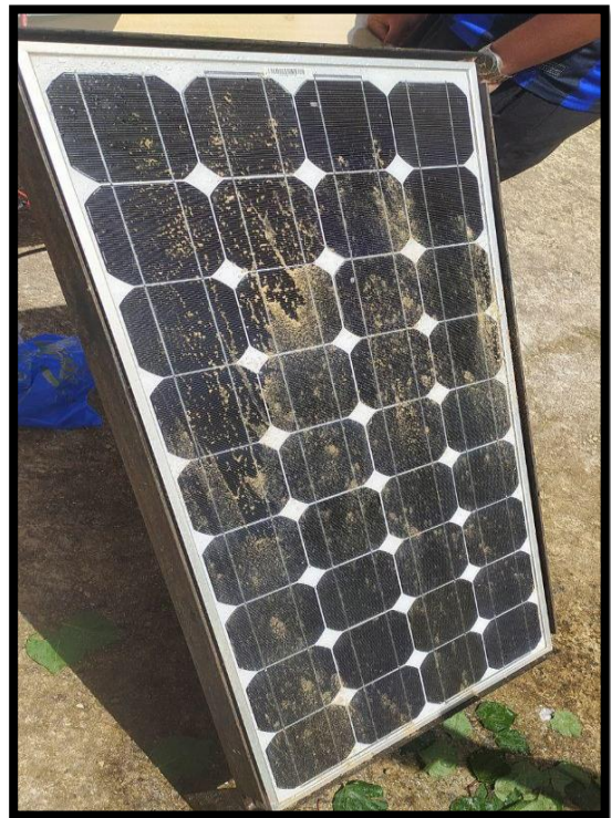
Figure III.1(h): The solar panel is covered with sand
