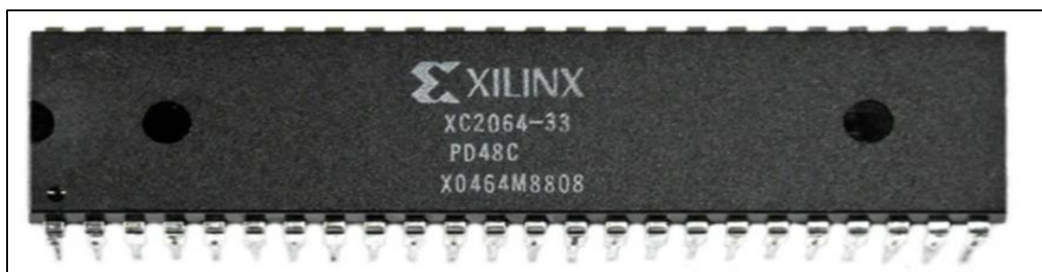
Figure II. 2: The first FPGA card (XC2064).
