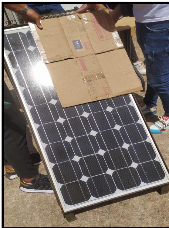
Figure III. 1(c): The solar panel is shaded 34%
