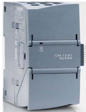
Figure II.17: Les Modules de Communication CM [18].
