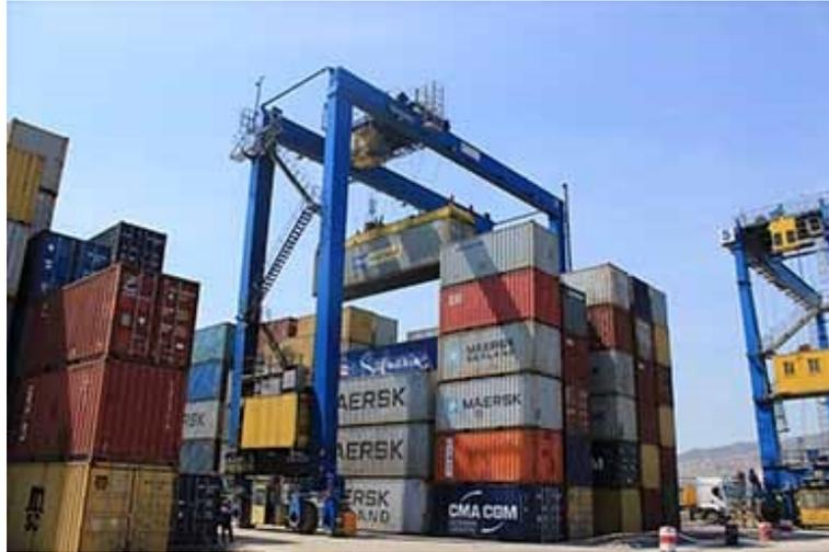
FIGURE 1.4 – RTG - Rubber-Tyred Gantry
