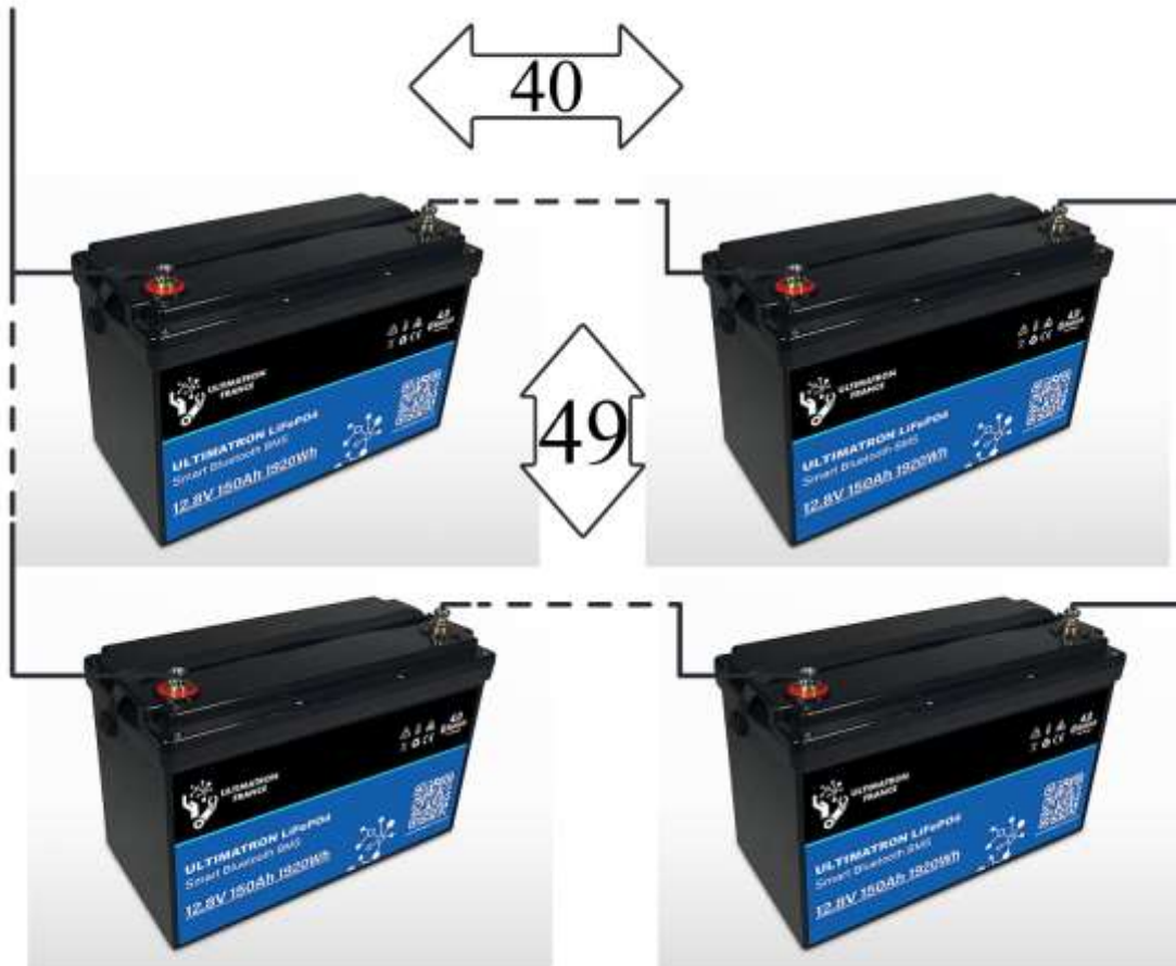
Figure II.17: Montage des batteries.
