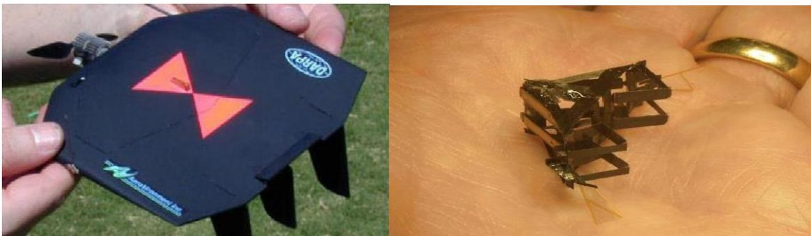
**Figure I.3:** Micro drones: Black Widow (Aerovironment, 42g) et Micromechanical Flying Insect (UC Berkeley, 25mm).
