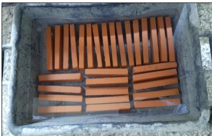
Figure II.36 : Briques (Sugar scum) immergés
