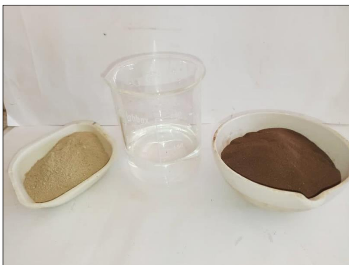
Figure II.23 : Mélange (argile +sugar scum+ eau)
