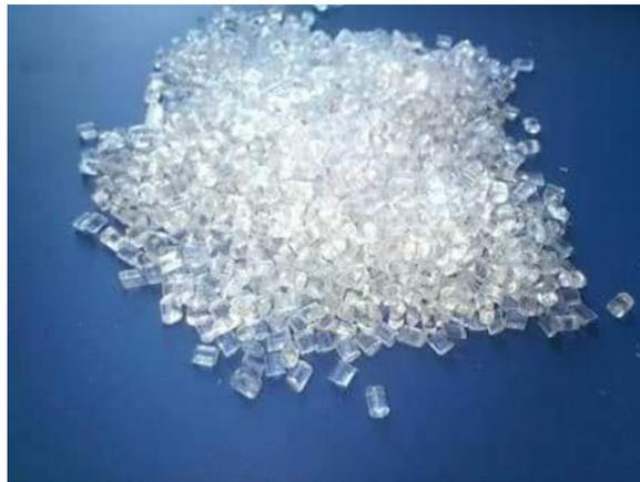
**Figure I.5.** Polystyrène cristal [20].
