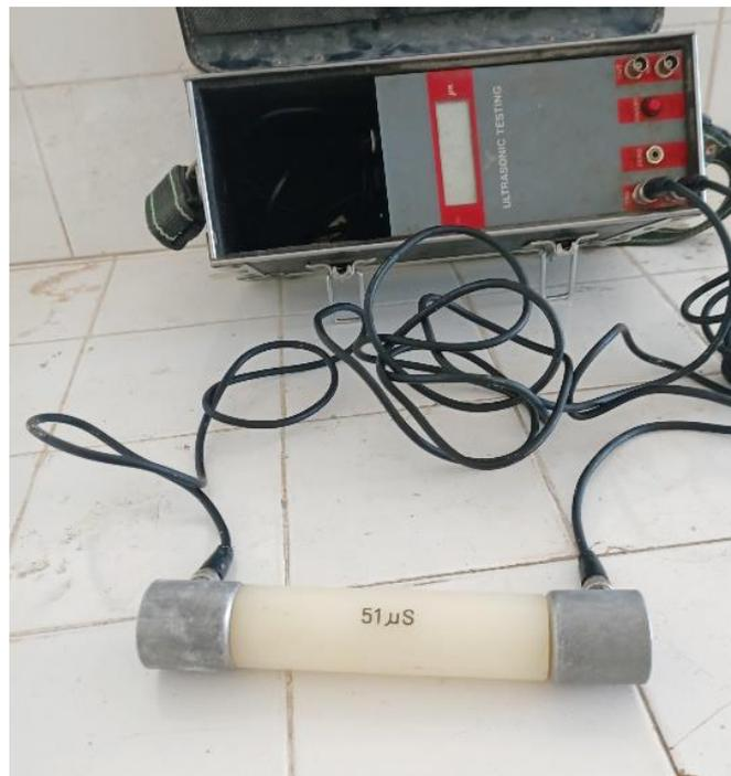
**Figure II.13.**Appareil Essai Ultrason
