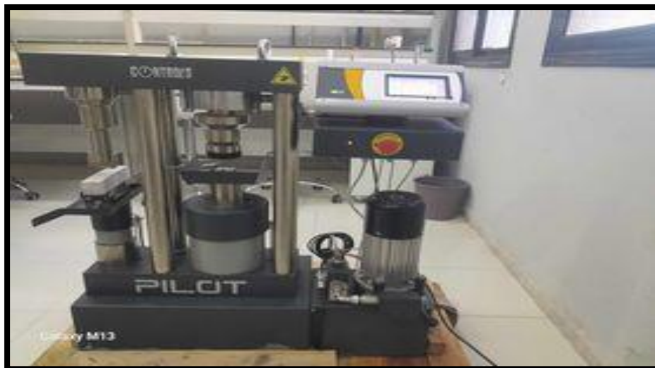
Figure II-17: Appareil de flexion (traction) compression.
