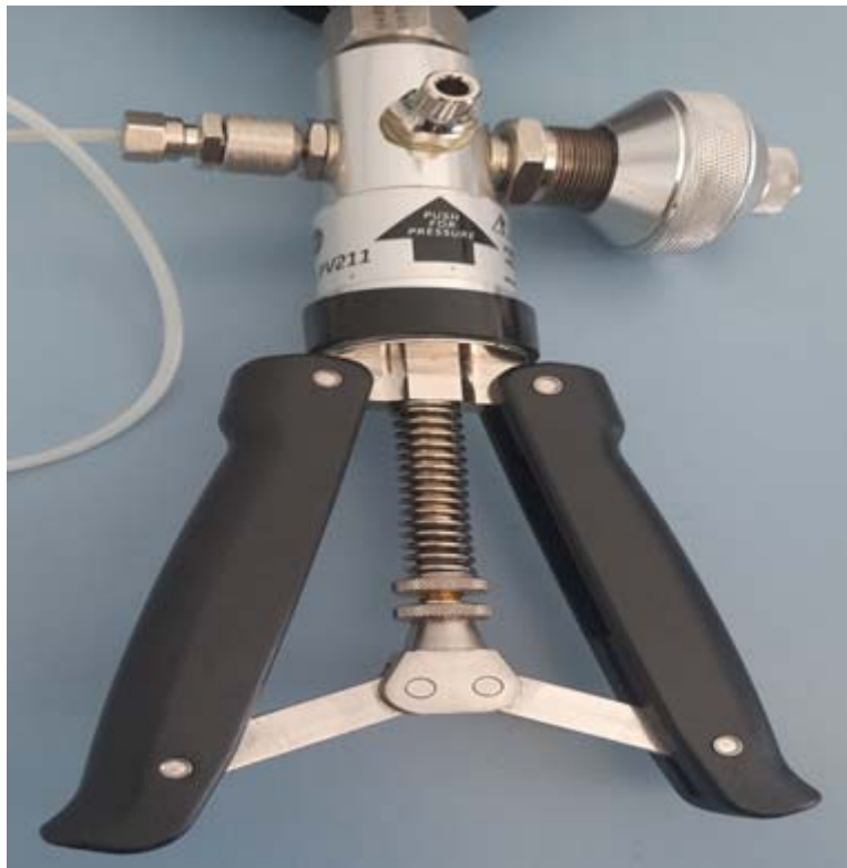
Figure III.17 : Pompe de pression.
