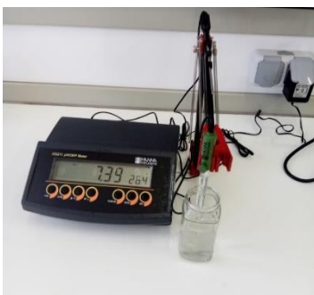
The pH meter (( \pm 0.01 precision)).
