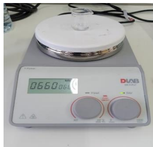
Magnetic stirrer Used for homogenization of mixtures. Also used during synthesis at room temperature.
