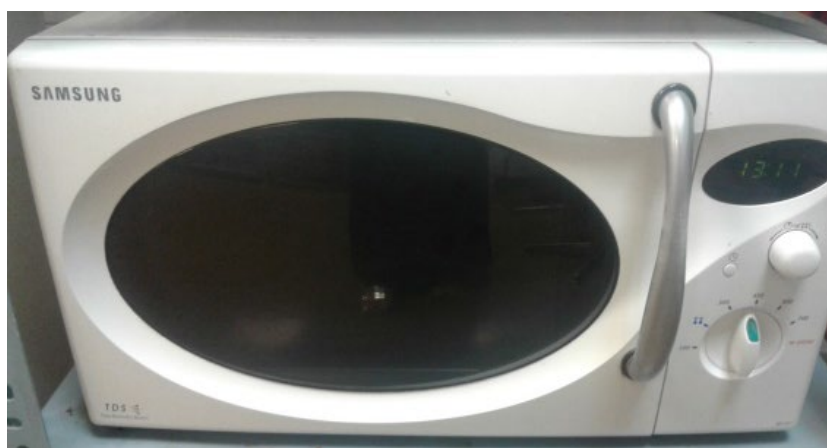
Figure 15. Microwave used to perform experiments on bacterial destruction (Samsung M1727, 2450 MHz)
