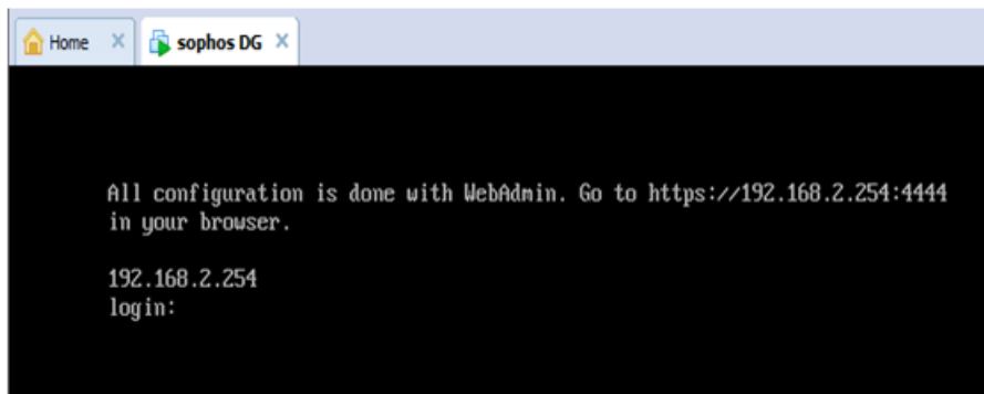
FIGURE 4.3 – installation terminé de la machine sophos DG.
