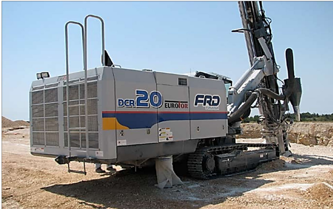
Figure III.2 : la sondeuse Furukawa FRD DCR-20.
