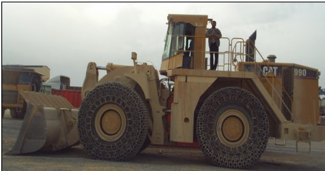
Figure II.5 Chargeuse CARTER PILAR 990. [11]
