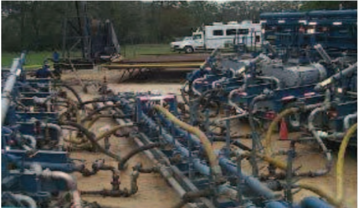
Rig up of a Manifold Trailer
