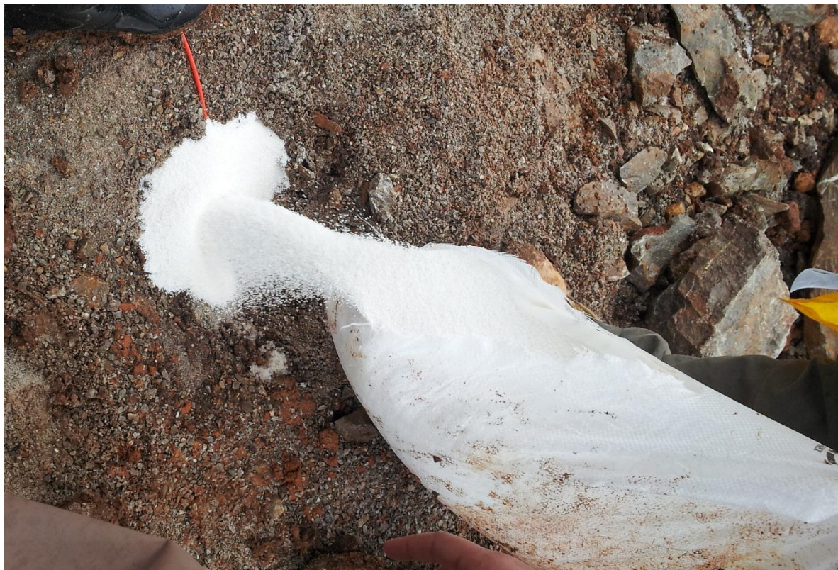
Figure III.2 : Explosif en vrac (Anfomil)
