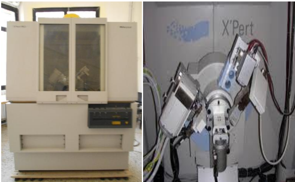
Figure III.1: Diffractomètre de marque Expert prof analytical type MPD / système vertical / .
