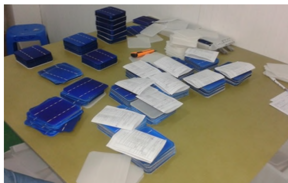
Figure II.10: Triage visuel des cellules
