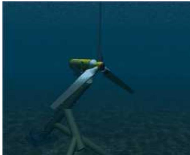
*Figure I.5* hydroliennes de type Hammerfest Strom AS.
