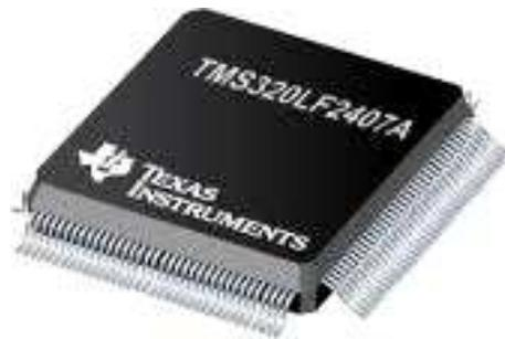
**Fig III.1.** Le DSP TMS320LF2407A
