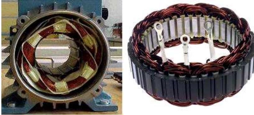
**Fig I.3.** Stator de la machine asynchrone
