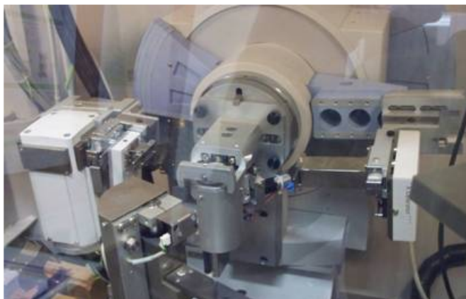
FIGURE 2.7 – Diffractomètre Theta-Theta PANalytical X'Pert Pro
